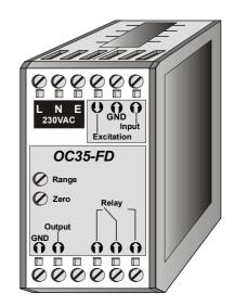
The Transmitter OC35-FD offers a five digit programmable divider with output transistor or mechanical relay. Depending on the setting of the divider, output pulses are generated after each liter, gallon, kg, pound etc. The transmitter delivers the momentary flow rate and the cummulated flow units at the same time.
